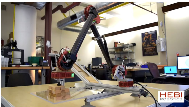
HEBI Robotics: Modular series elastic actuators (SEAs).
