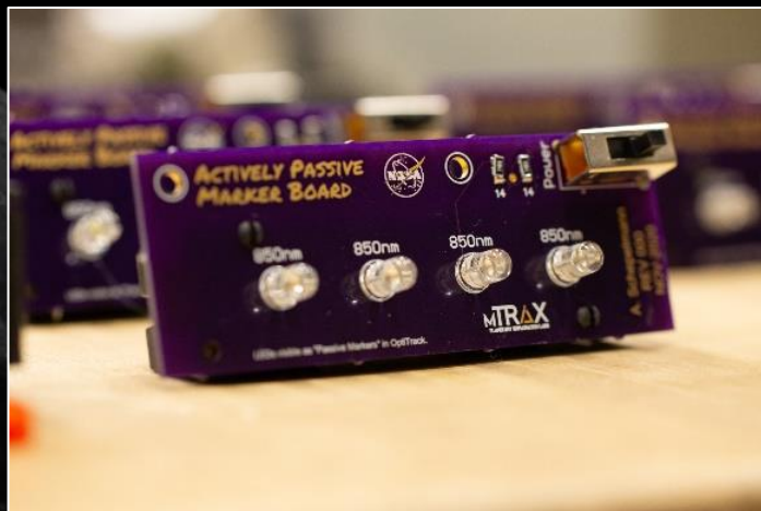
Figure 5. Actively passive marker board designed and built by the mTRAX team.
