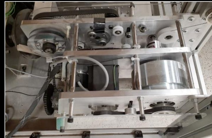
Figure 12. Fully installed drawbar pull rig.
