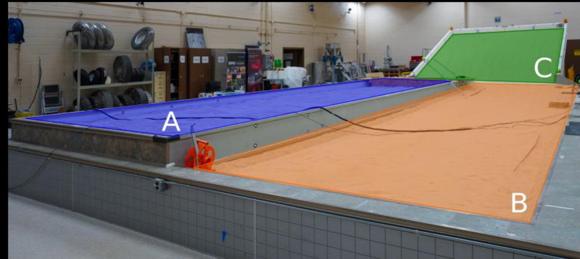
Figure 2. SLOPE laboratory soil bins. A: High-sinkage Fillite. B: GRC-1. C: Tiltbed.
