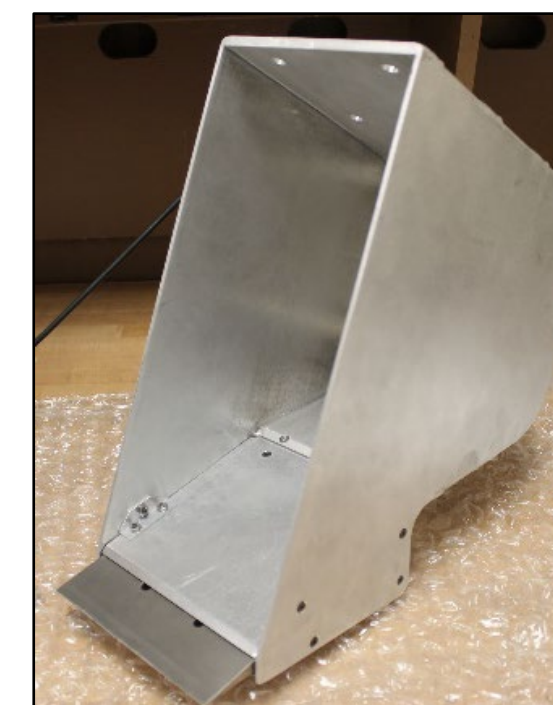
Figure 3: Ultrasonic bucket with integrated 20 kHz vibrating leading edge.
