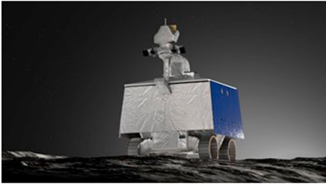
Figure 1. Rendering of VIPER on the lunar surface. The rover measures 2.5 m tall and 1.5 m in length and width.
