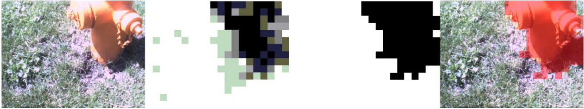
FIGURE 33: Full image processing with a fire hydrant obstacle. (Left to right) Input image, pre-thresholded voting combination, generated binary freespace, overlay of input image and freespace.
