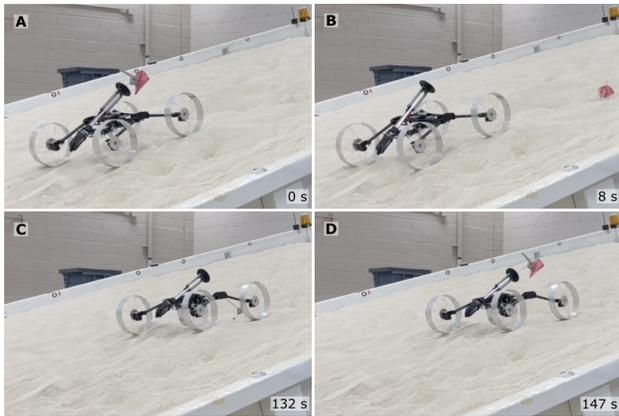
Fig. 10. The anchor launcher being used to climb a  $17^\circ$  slope of GRC-1 lunar regolith simulant at the NASA Glenn Research Center SLOPE Lab. A) Rover is stuck and cannot climb further. B) Anchor is launched. C) Rover has winched itself up to anchor. D) Anchor is pulled out of sand and resets into launcher.
