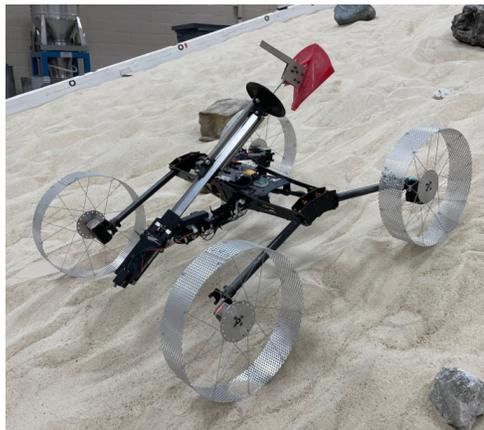
Fig. 1. The anchor launcher mounted on a rover mobility platform to help climb a 17° slope of loose regolith simulant at the NASA Glenn Research Center SLOPE Lab. For scale, the rover wheel base is 57 cm long.
