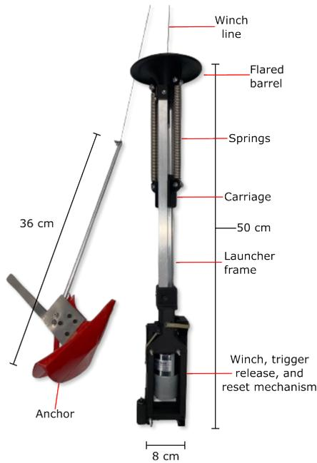
Fig. 2. The anchor, on the left, connected by the winch string to the launcher, on the right.
