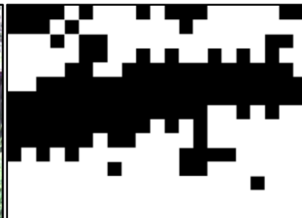
Fig. 9. Segmentation results of Fig. 8 based on horizontal binary variance statistics for 31x31 neighborhoods. This statistic recognizes the majority of illuminated and shaded grass as driveable terrain (white regions), while marking the flowerbed edging and some flower buds at the top of the image as obstacle containing (black).
