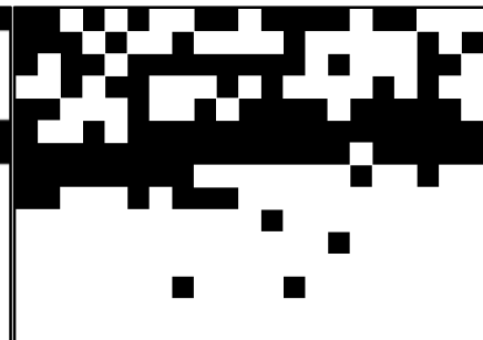
Fig. 10. Segmentation results of Fig. 8 based on binary centroid location of illuminated grass for 31x31 neighborhoods. This statistic also recognizes grass as driveable terrain (white regions), while marking the flowerbed edging and many flower buds as obstacles (black).
