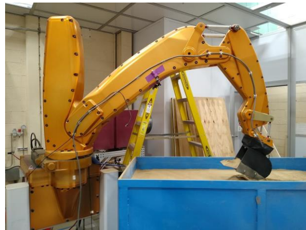
Figure 1. The APEX excavation platform in the Excavation Lab at NASA Glenn Research Center with the first generation Ultrasonic Bucket prototype attached as the end effector.
